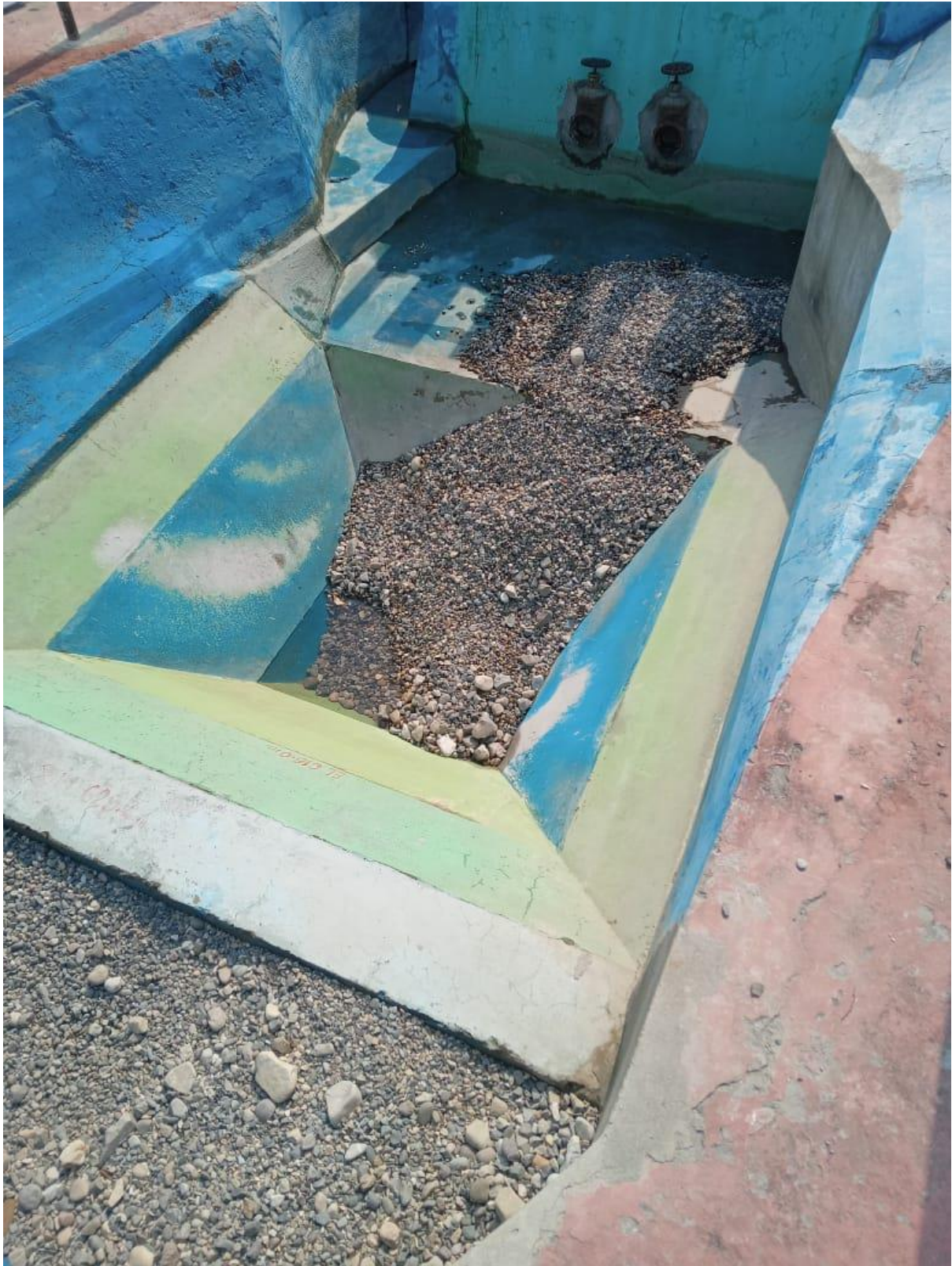
Photo 24: Scouring within Plunge pool and downstream of end sill in river at 7590 \text{ m}^3/\text{s} while only 4 gates were open (free flow)
