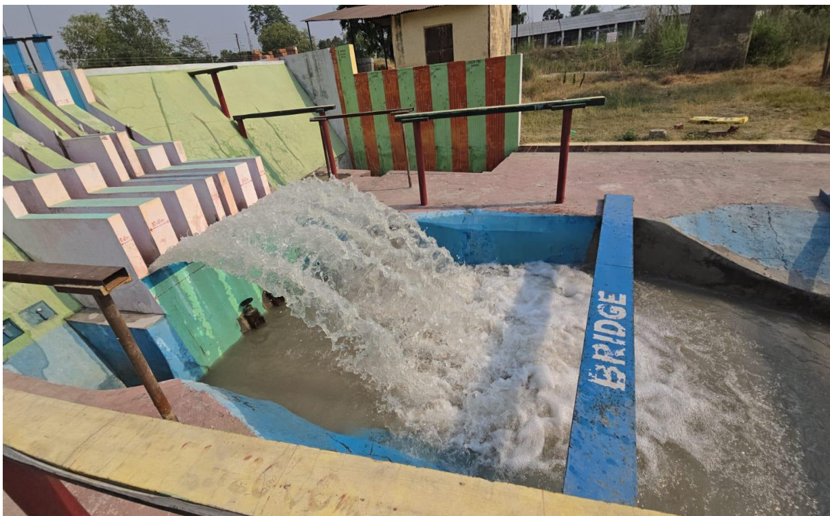
Photo 19: Flow behaviour of jet trajectory and plunge pool at HFL at 2 m gated condition
