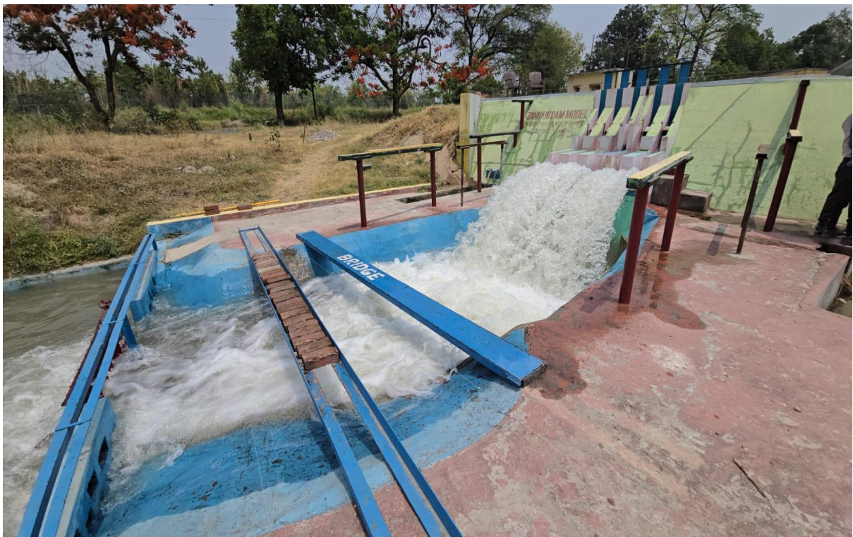
Photo 13: Flow behaviour of jet trajectory and plunge pool while all 5 gates open at HFL at free flow
