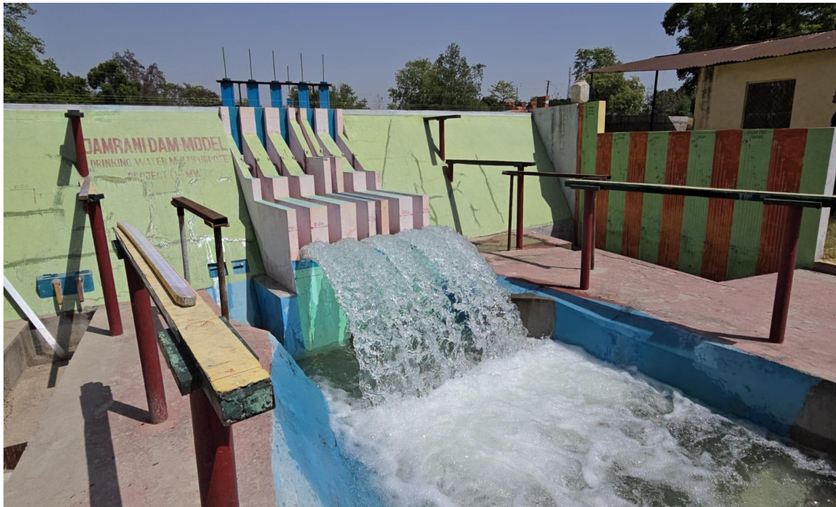
Photo 10: 5 Flow behaviour of jet trajectory and plunge pool while all 5 gates open at 3800 \text{ m}^3/\text{s} at free flow
