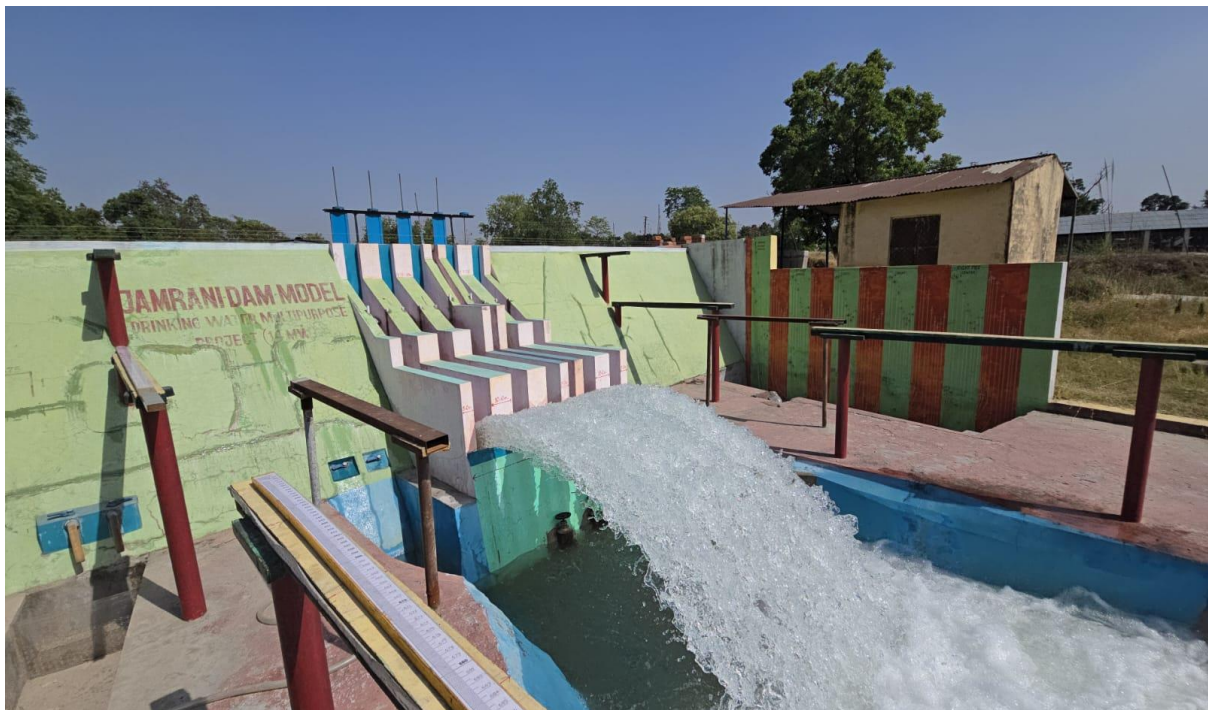
Photo 11: Flow behaviour of jet trajectory and plunge pool while all 5 gates open at 5700 \text{ m}^3/\text{s} at free flow
