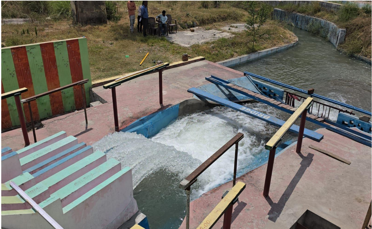
Photo 16: Flow behaviour of jet trajectory and plunge pool while all 4 gates open at 5700 \text{ m}^3/\text{s} at free flow
