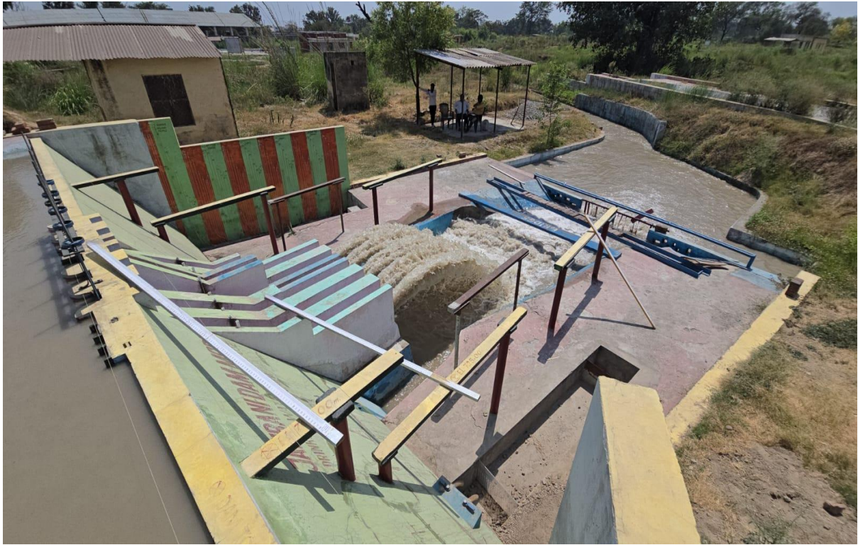
Photo 08: Flow behaviour at upstream of dam axis at 9 m equal gate opening of all 5 bays at HFL
