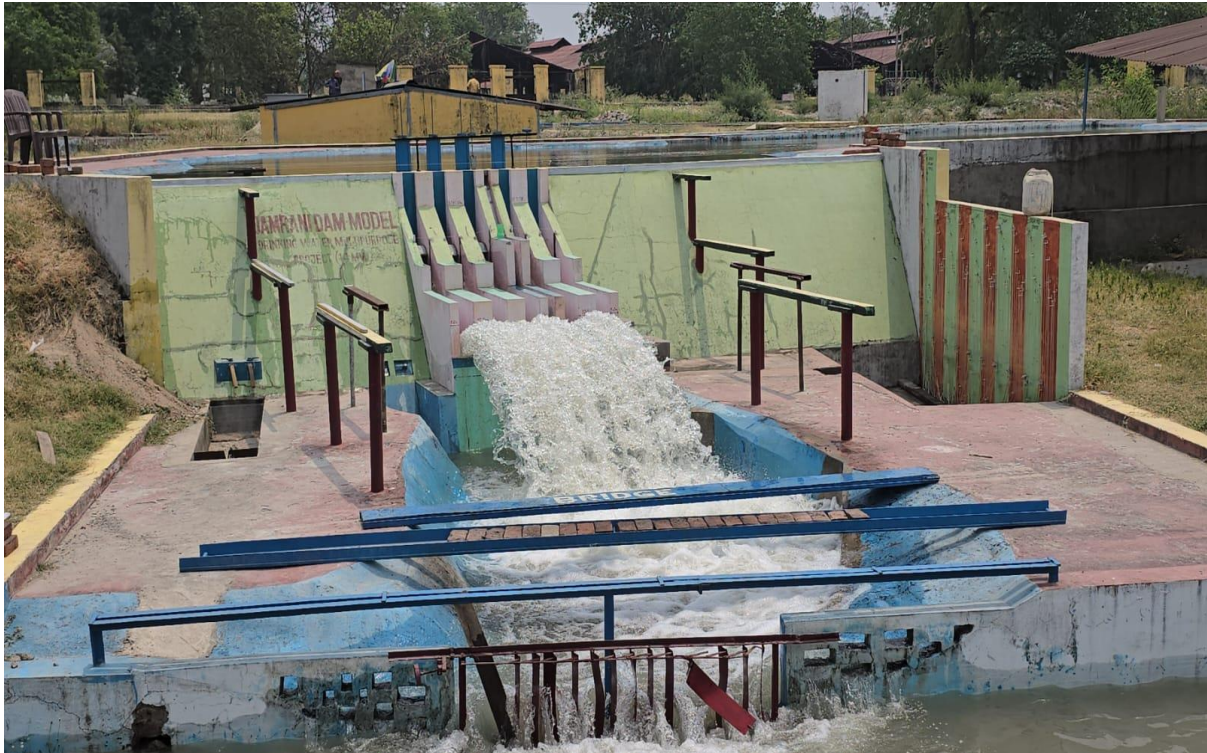
Photo 18: Flow behaviour of jet trajectory and plunge pool while 4 gates open at HFL at free flow
