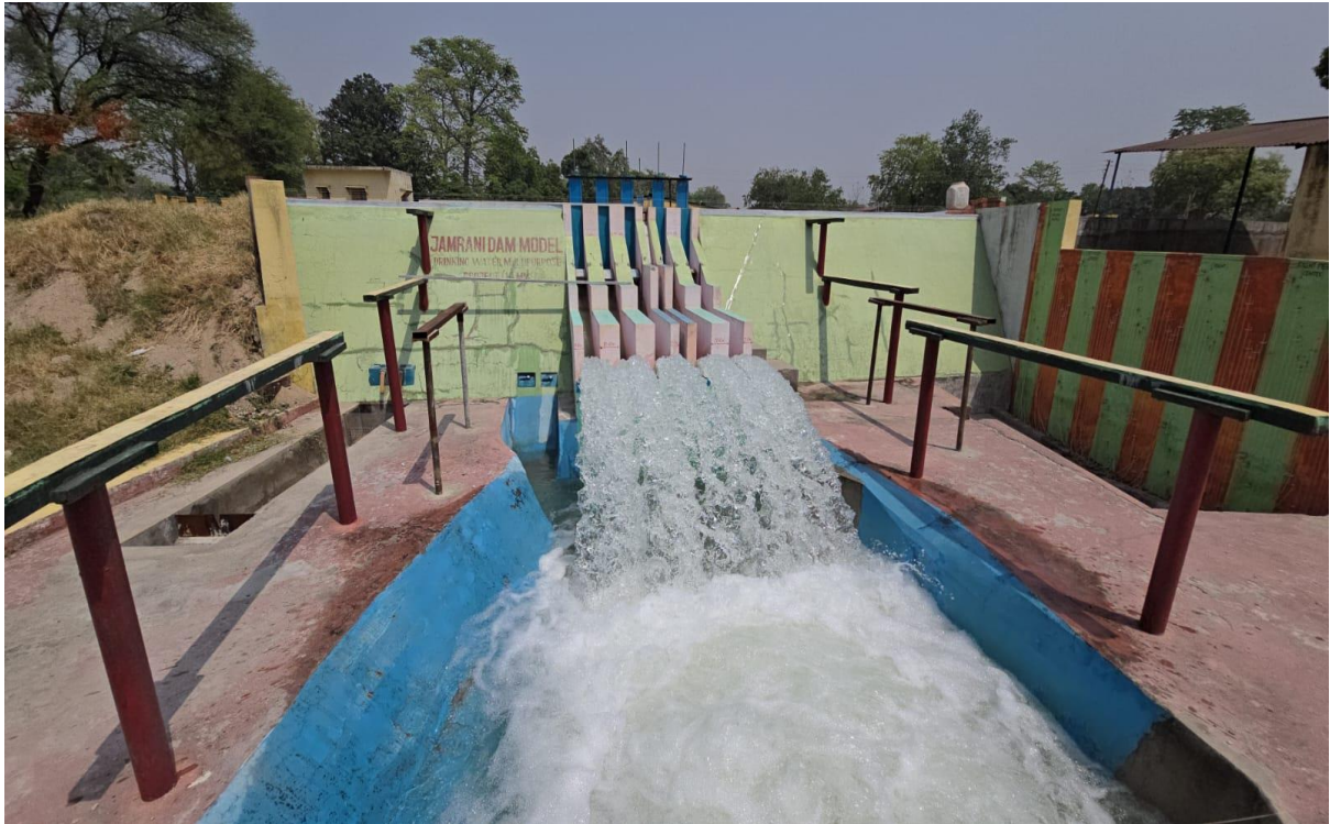
Photo 12: Flow behaviour of jet trajectory and plunge pool while all 5 gates open at 7590 m 3 /s at free flow
