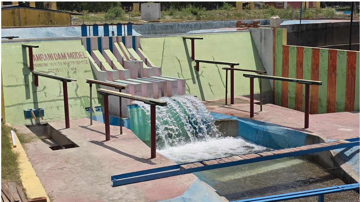
Photo 09: Flow behaviour of jet trajectory and plunge pool while all 5 gates open at 1900 \text{ m}^3/\text{s} at free flow
