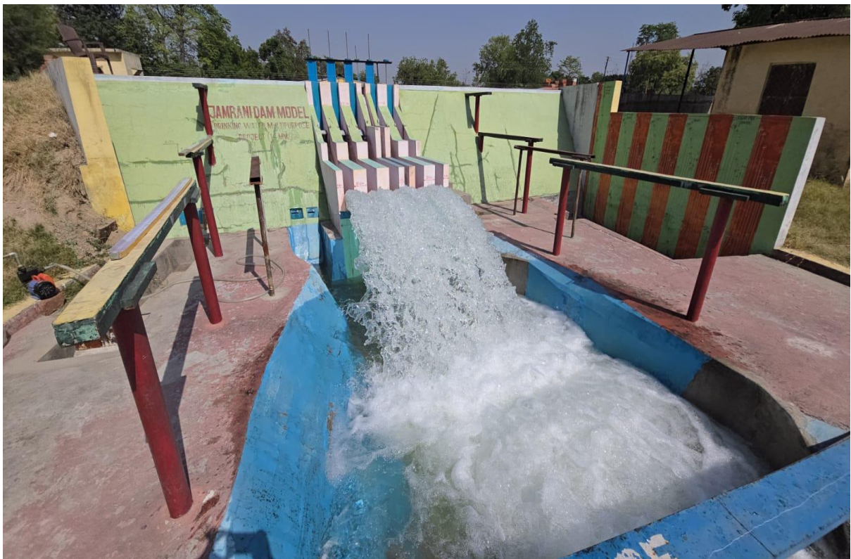
Photo 17: Flow behaviour of jet trajectory and plunge pool while 4 gates open at 7590 \text{ m}^3/\text{s} at free flow
