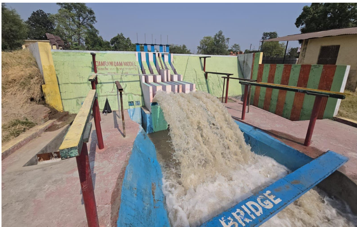
Photo 20: Flow behaviour of jet trajectory and plunge pool at HFL at 6 m gated condition
