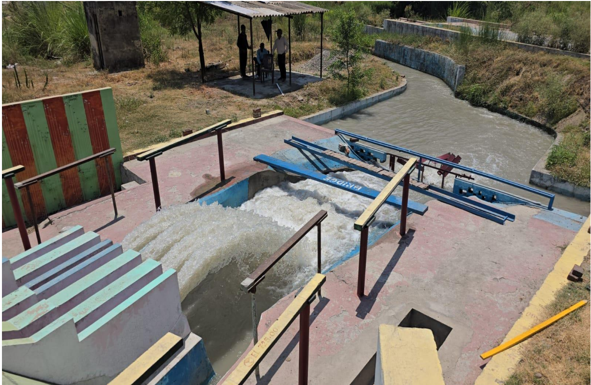
Photo 22: Flow behaviour of jet trajectory and plunge pool at HFL when only 4 bays 9 m open gated condition at HFL
