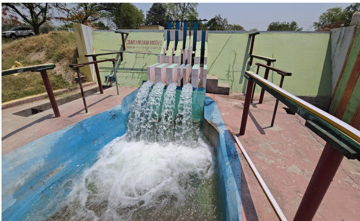
Photo 14: Flow behaviour of jet trajectory and plunge pool while 4 gates open at 1900 \text{ m}^3/\text{s} at free flow
