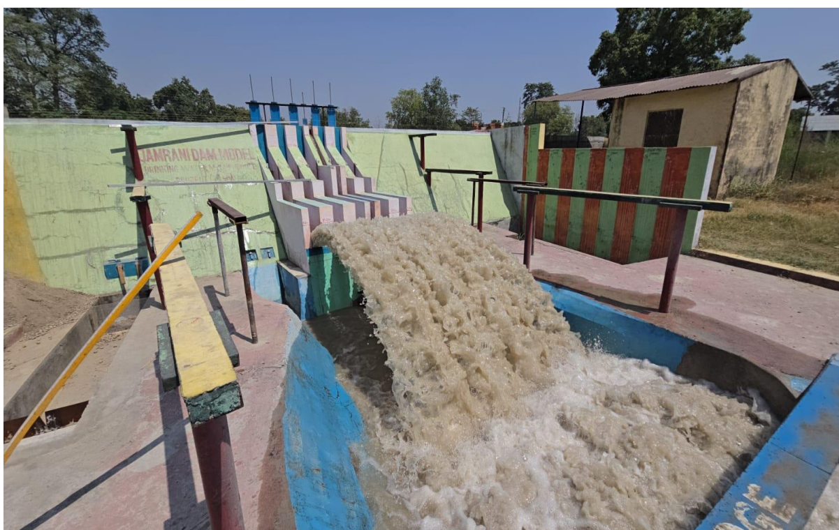
Photo 21: Flow behaviour of jet trajectory and plunge pool at HFL at 8 m gated condition
